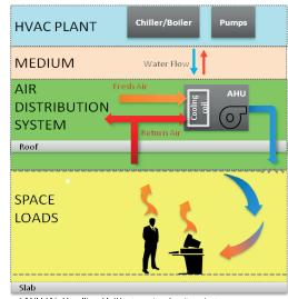
\* AHU (Air Handling Unit): air cooling/heating device
